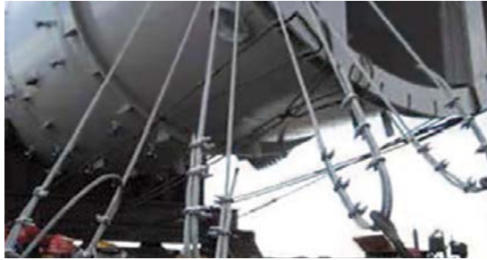
Wire lashing arrangements offer extra insurance against cargo movement.
