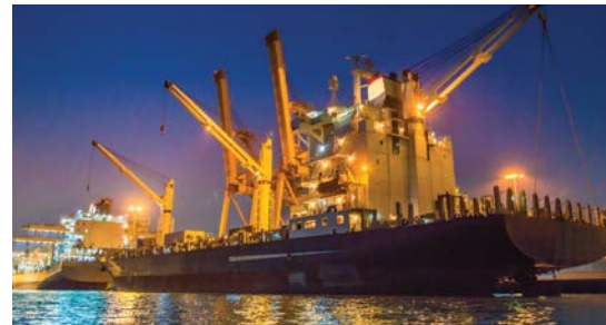
A heavy-lift vessel specifically designed for the carriage of heavy project cargo. Two cranes allow for tandem lifts.
