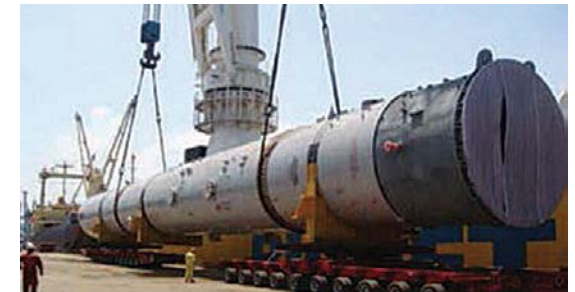
A tandem lift compensates for an off-centre CoG.
