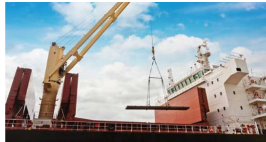
A single, heavy-lift derrick on a cargo vessel poses limitations on the lifting of long columns.
